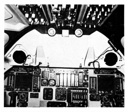
BLACK CIRCLES are thermal flashblindness protective windows mounted in the cockpit of the Air Force's B-1B aircraft. The Sandia-invented electrooptic ceramic PLZT darkens the windows much faster than a human blink to exclude 99.9 percent of any sudden light or thermal energy.
